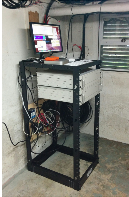
Illustration 2: The CODAR electronics at Georgina Point. The entire system uses less than 500 Watts of power.
