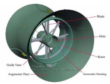
0-1 Imagine of the tidal current turbine generator installed at Race Rocks[6]
